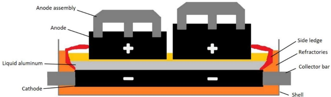
**Figure 1. Electrolysis cell main components.**
